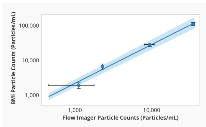
**FIGURE 4:** Comparison of HORIZON<sup>®</sup> and flow imager IgG particle counts. Both systems showed a linear response, but the HORIZON<sup>®</sup> system demonstrated increased sensitivity, detecting 3.26X more particles compared to flow imager for this formulation. 95% confidence interval of the linear fit (light blue).
