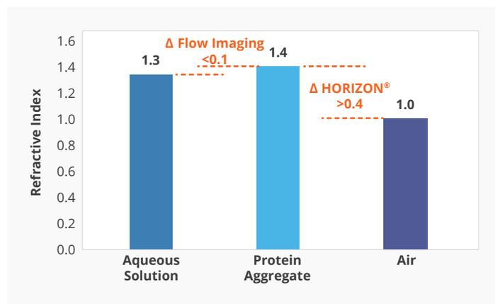
**FIGURE 3:** Refractive index differences between protein aggregates in aqueous solutions (FI) and air (HORIZON<sup>®</sup>). The higher refractive index contrast with the HORIZON<sup>®</sup> system improves data accuracy, robustness, and sensitivity.
